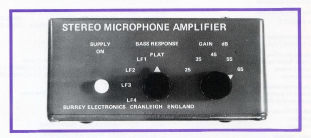
The Stereo Microphone Amplifier takes inputs from 50 or 200 Ohm microphones and offers good noise and input loading characteristics by a series-parallel arrangement on the transformer primary. The gain is variable in five 10dB steps and a choice of four low frequency roll-off curves is available in addition to a flat response position. Low frequency attenuation is often useful in improving the clarity of recordings and the various curves available are shown in the graph.
