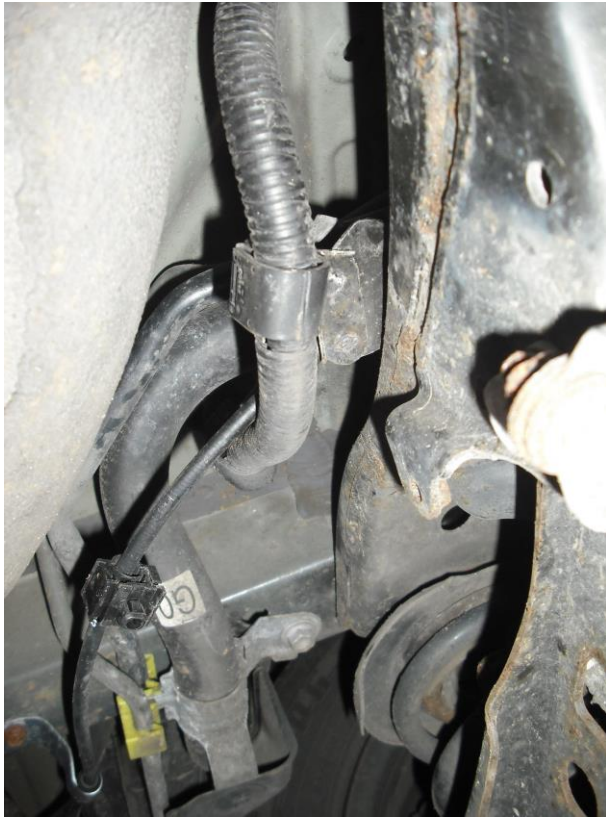
Manual parking brake release Bowden cable descending from the rear boot area:
