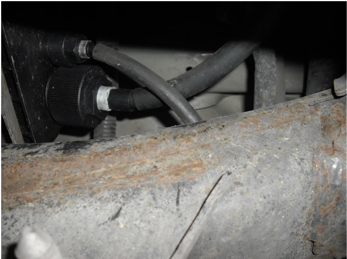
Parking brake release Bowden cable and a brake actuator connected to the EPB:
