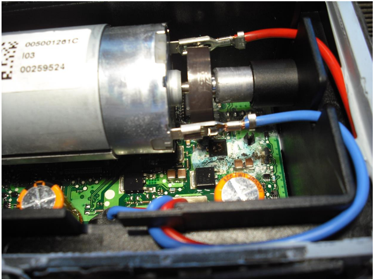
White corrosion salts on the circuit board below the manual parking brake release:
