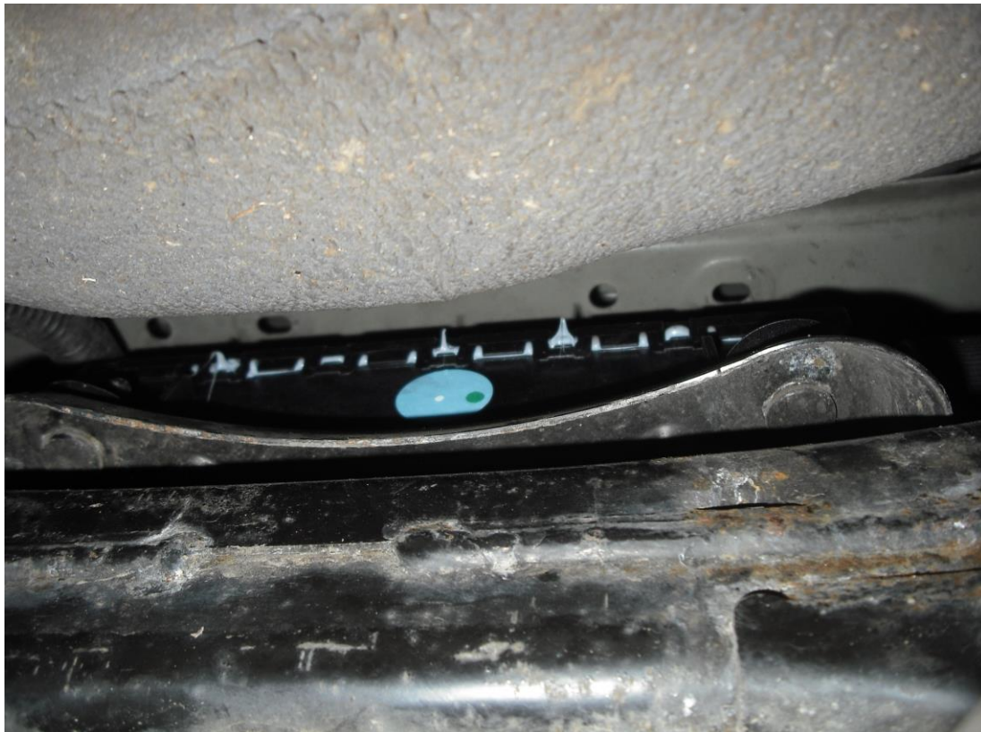
Electronic Parking Brake mounted above a strut between the rear wheels:
